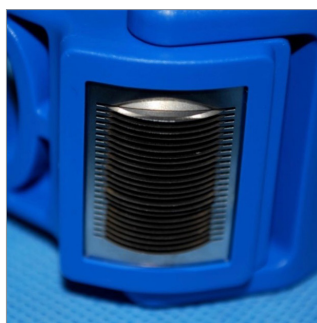
Figure 1. A close up of the cutting discs that simultaneously hold and cut the skin in the mincer device.
